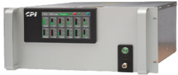
CPI 1250 W Ku-band TouchPower TWTA, Model T5UI-12
